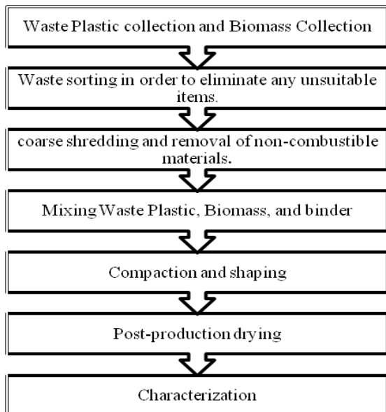
Figure 5: Flow Diagram of Waste Plastic-Biomass Briquette Manufacturing Process.
